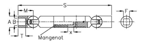
$A = 45 \\ F = 22 \\ Longitudinal ribs = 6x21x25 \\ M = 55.0 \\ MD max N m = 200 \\ s = 400 \\ T = 26 \\ x = 140$
